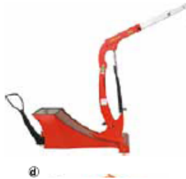
Counterweight crane with large free jib in front of the wheels (modern design)
